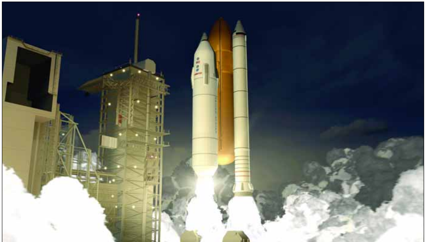
One of the most-discussed heavy-lift launch vehicle concepts is based upon using a variety of shuttle-derived components, such as this notional Shuttle-C design. (Source: NASA/John Frassanito & Associates)
